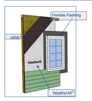
WeatherAll® must not contact hot objects (e.g. chimneys, furnace and water heater flues, lighting fixtures, etc.) be sure to conform to local building codes when installing.
