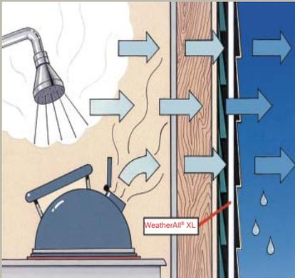
We put over 1,000 vapor holes\* in every square foot of WeatherAll®. These tiny holes enhance water vapor permeability. This important feature helps ensure that water vapor can escape the wall cavity. Trapped water vapor can cause mold formation and, if unnoticed, can lead to structural damage.
